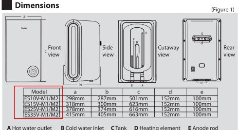
A Hot water outlet **B** Cold water inlet **C** Tank **D** Heating element **E** Anode rod **F** Thermometer tube **G** Wall-mounting bracket **H** Temperature regulating knob **Remarks:** 1. The permitted error limit of the above parameters is ±10%.
